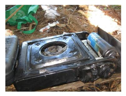
Overheating will also occur if the cooking vessel, for example a pot, frying pan or baking tray, is larger than the canister cooker was designed for. Even if the pot supports are the right way up, an over-large cooking vessel will direct heat towards the canister compartment and may cause the canister to overheat.
