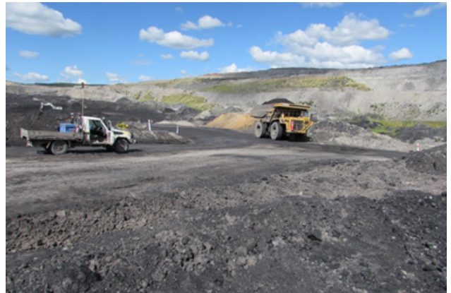
FIGURE 6: Near-miss incident. Light Vehicle at approximate position where it stopped to avoid the truck. Truck at approximate position it had slowed before entering intersection. Note: Give way sign obscured by truck
