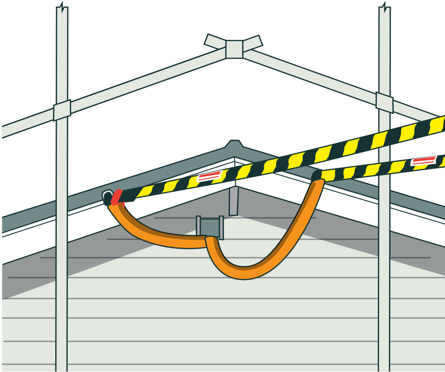
FIGURE 7: A combination of tiger tails and insulated covering
