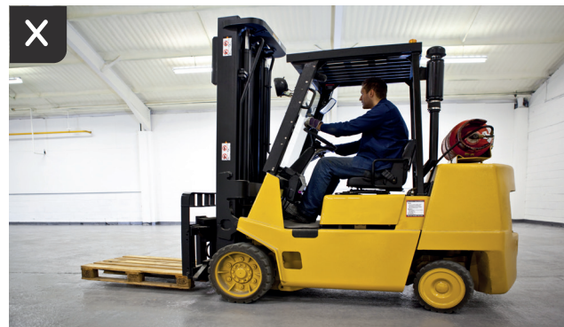
FIGURE 1: Avoid using LPG and other fuel-powered forklifts in coolstores and areas with poor ventilation
