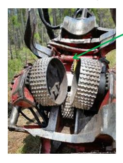
Operator trapped between feed rollers
