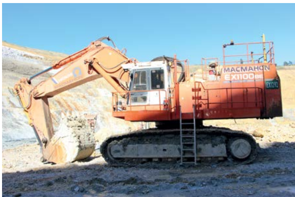
Figure 13: This excavator has a good access system, with platforms, guardrails, kick plates and ladder. The ladder is interlocked so the vehicle cannot be started without the ladder being raised
