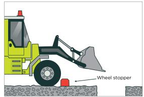
Figure 46: Prevent plant operation near excavations
