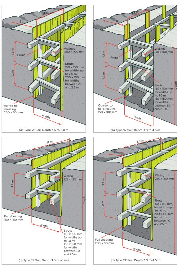
Figure 37: Timber shoring requirements for trenches
