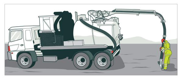
Figure 42: Vacuum truck digging a pilot hole
