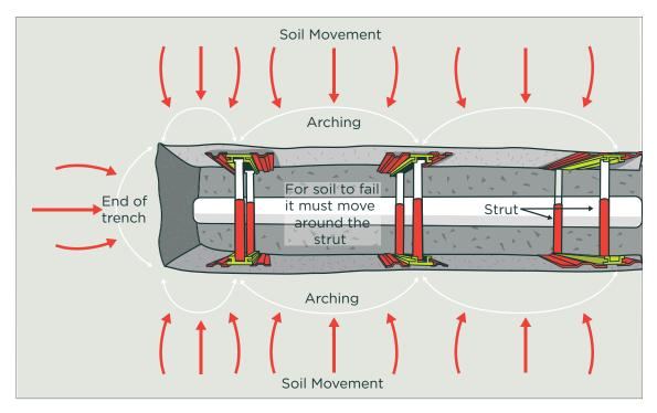
Figure 24: Hydraulic soldier shoring using soil arching
