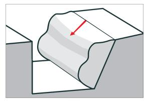
Figure 17: Subsidence and bulging
