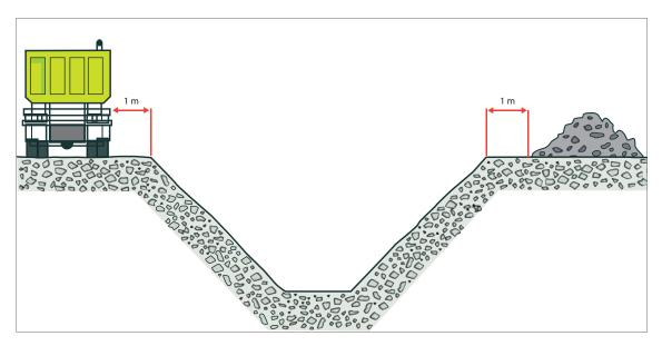
Figure 21: Battering control
