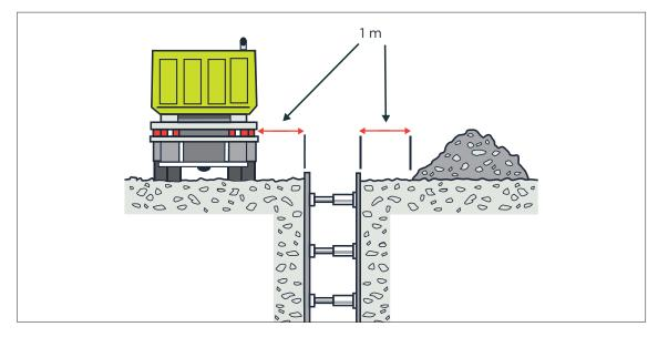
Figure 39: A shored excavation designed to carry soil, vehicle and spoil loads
