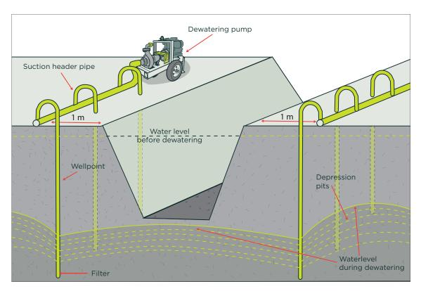
Figure 45: Use well point pumping for lowering groundwater by up to 6 m
