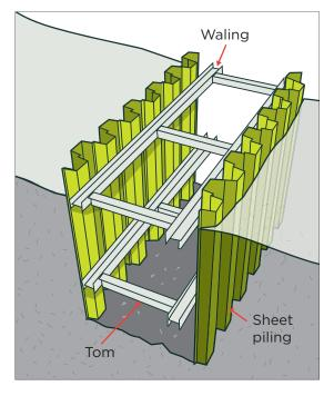
**Figure 29:** Steel sheet piling with internal waling support
