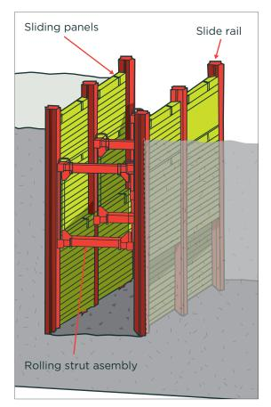
Figure 28: Slide-rail or rolling-strut shoring
