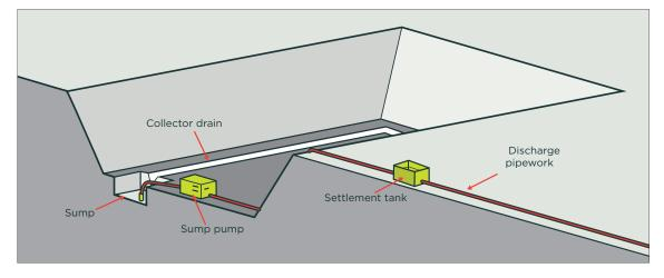
Figure 44: Traditional sump pumps control surface water at the excavation's base
