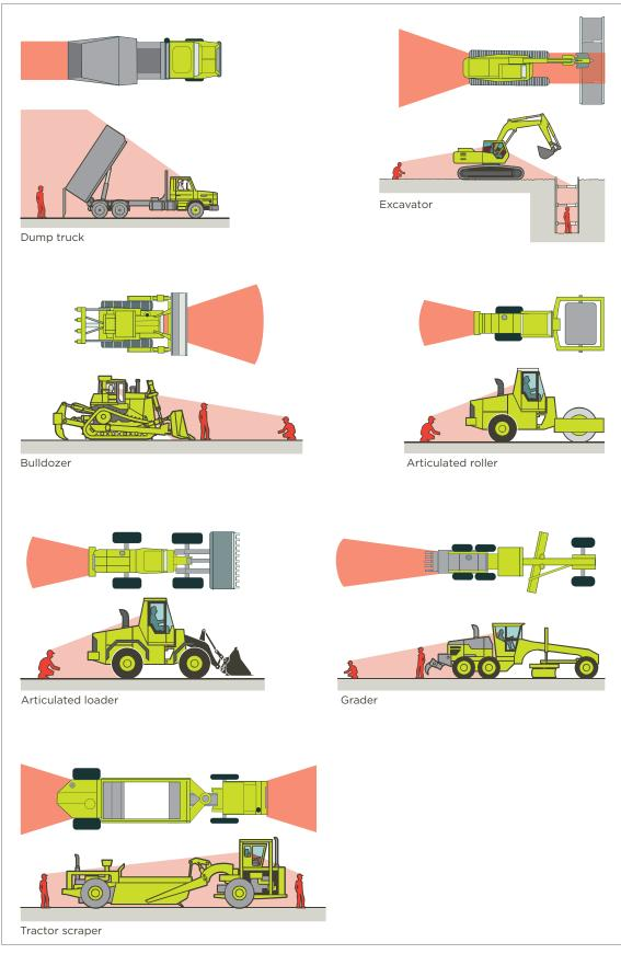
Figure 48: Mobile plant operator blind spots
