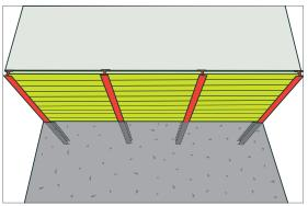
Figure 34: H-pile shoring with timber lagging
