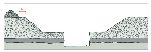
Figure 22: Combination of benching and battering controls
