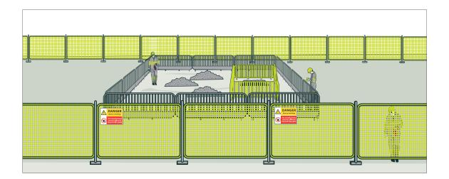
Figure 13: Externally fenced site with internal fences
