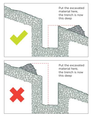
**Figure 40:** Spoil placement on effective excavation depth
