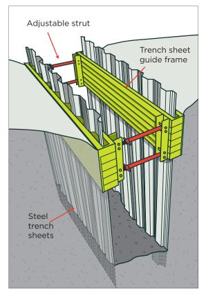
Figure 30: Guide framed steel trench sheeting
