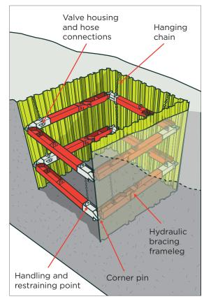
**Figure 33:** Hydraulic bracing frame with steel trench sheeting
