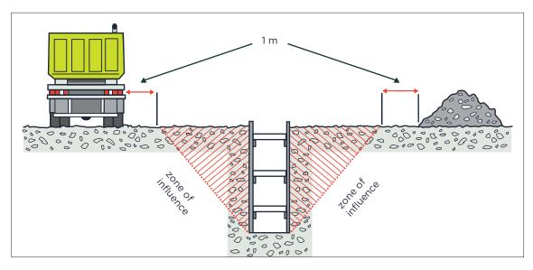
Figure 38: A shored excavation designed to carry soil loads only
