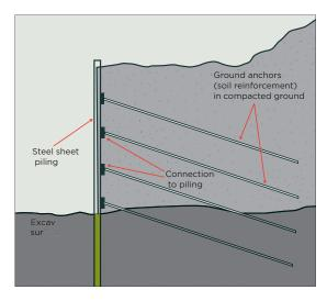
Figure 31: Ground anchors for supporting steel sheet piling
