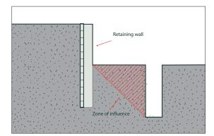
Figure 12: Retaining wall restriction
