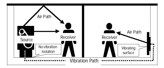
Noise can be controlled at the point of **source**, by blocking the **noise path**, or protecting the **receiver**. Noise control options centred on the noise source are the most effective, while noise control options centred on protecting the receiver are the least effective. Receiver-based options control exposure to noise rather than the noise itself.
