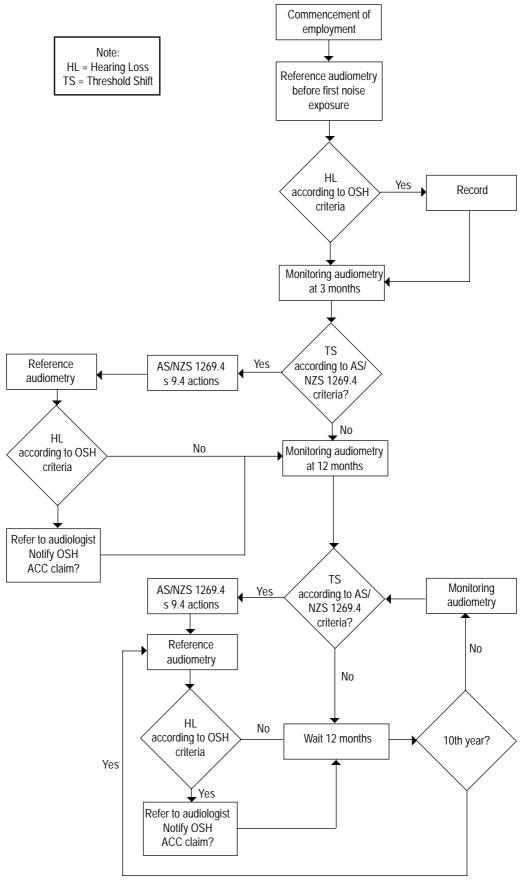
Figure E.2: Flow chart of audiometry testing procedure given in AS/NZS 1269.4
