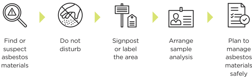
FIGURE 7: What to do if you find or suspect asbestos in your building
