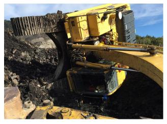
**INCIDENT 3:** An excavator crossed a small culvert onto unleveled ground with the bucket elevated, causing the excavator to tip over
