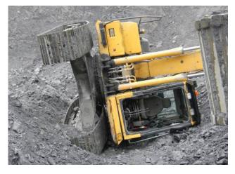
**INCIDENT 1:** The excavator tipped off the raised dirt platform from which it was loading trucks. The excavator moved to the ore stockpile pile to load another truck. One track was over the edge of the pile. The operator then slewed the machine to loadout, and the machine rolled when the weight transferred to the unsupported track
