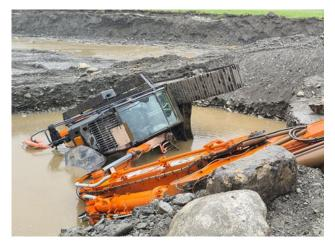
**INCIDENT 4:** The excavator was tramming beside a mine pond when the ground gave way. The excavator track dropped down and the excavator tipped into the pond
