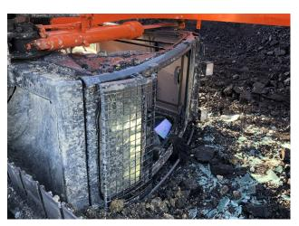
**INCIDENT 2:** The excavator tipped over a one-metre high face/canch. A lone operator had placed his tracks close to the canch edge and was trying to remove a parting. The bucket grabbed and pulled the excavator over the edge
