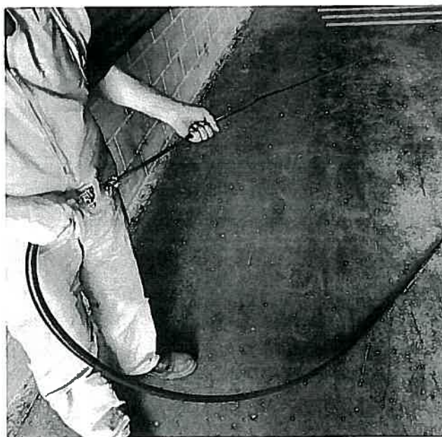
Figure 1: Air-Lance used to remove fibre build up
