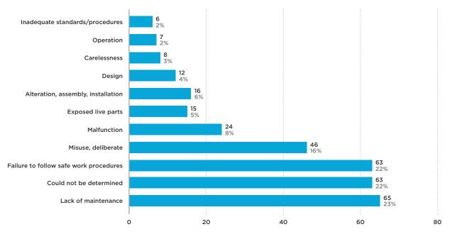
FIGURE 1D: Notifiable electrical accidents by causal factor
