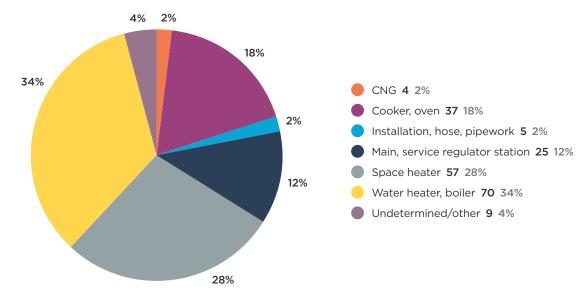
FIGURE 2E: Notifiable natural gas accidents by equipment
