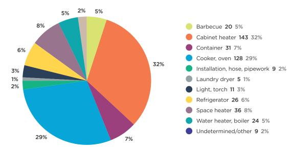
FIGURE 3E: Notifiable LPG accidents by equipment
