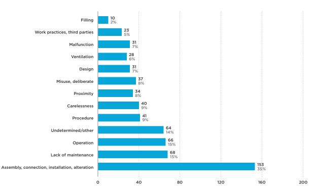
FIGURE 3C: Notifiable LPG accidents by causal factor
