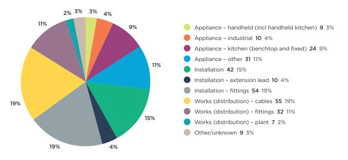
FIGURE 1E: Notifiable electrical accidents by equipment
