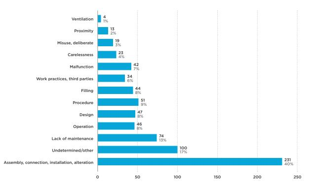
FIGURE 3D: Non-notifiable LPG accidents by causal factor
