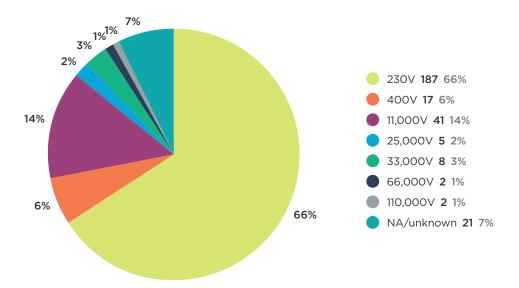
FIGURE 1C: Notifiable electrical accidents by voltages
