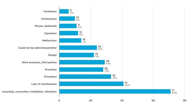
FIGURE 2C: Notifiable natural gas accidents by causal factor
