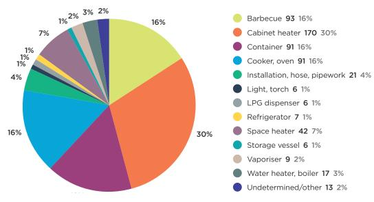
FIGURE 3F: Non-notifiable LPG accidents by equipment
