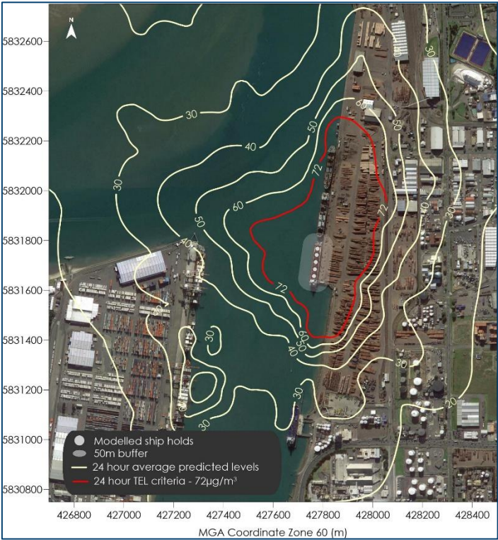
Figure B-56: Maximum predicted EDN concentrations ( \mu\text{g}/\text{m}^3 ) - Ship holds, 24-hour averages, 700ppm
