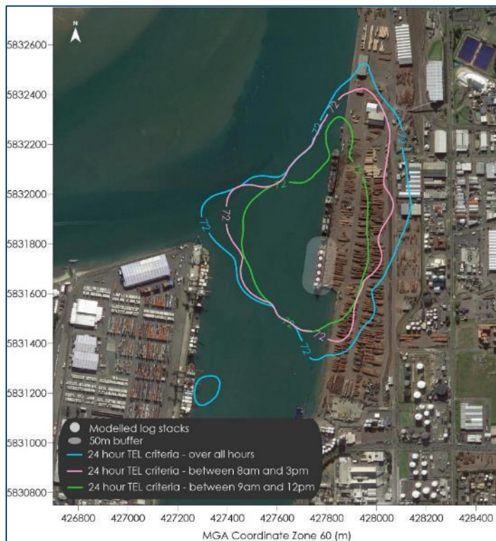
Figure 4-59: Maximum predicted EDN concentrations (µg/m³) - Ship holds, 24-hour averages, 1,000ppm, with ventilation across all hours, between 9am and 3pm and between 9am and 12pm
