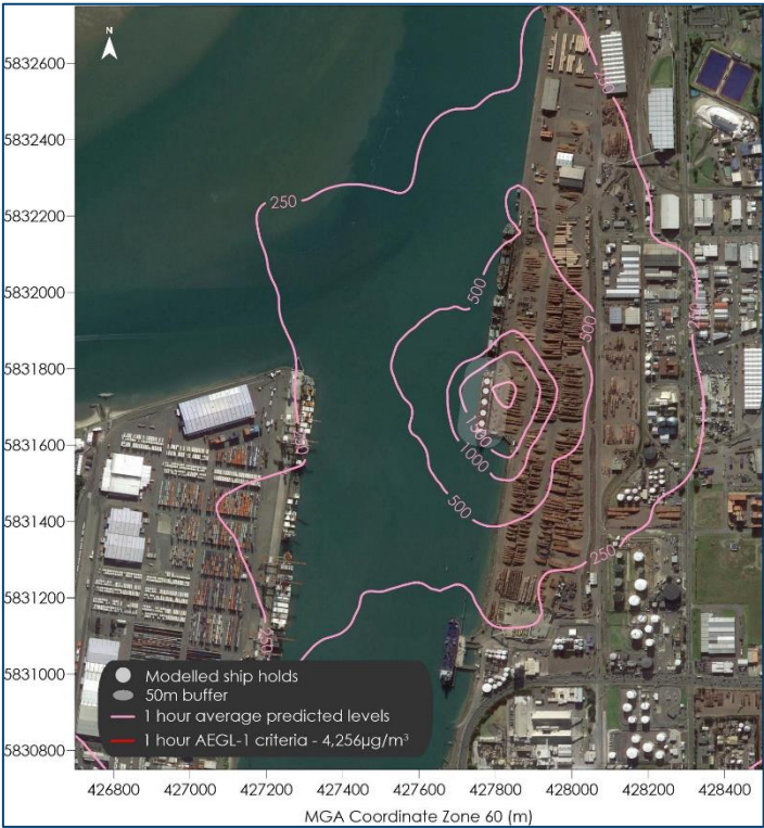
Figure B-50: Maximum predicted EDN concentrations ( \mu\text{g}/\text{m}^3 ) – Ship holds, 1-hour averages, 500ppm
