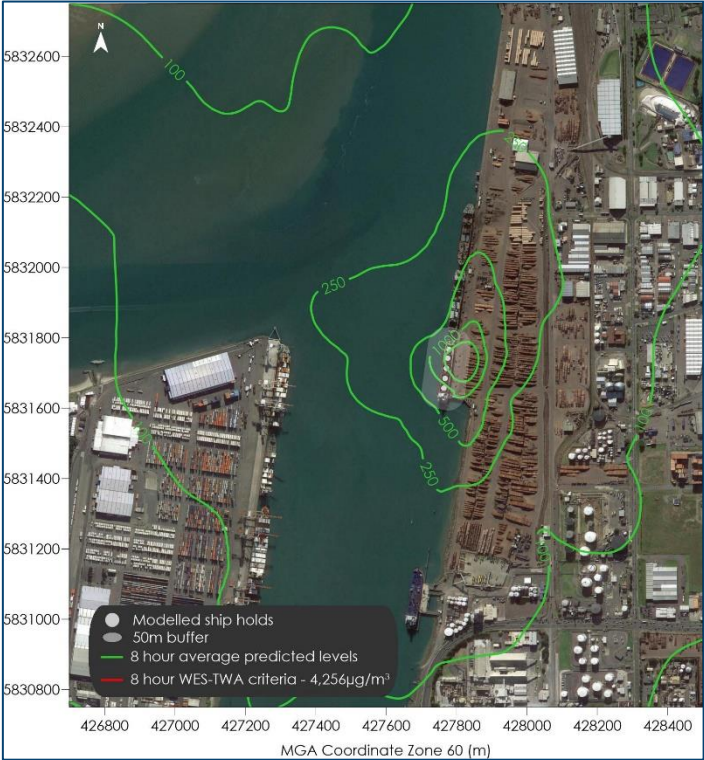
Figure B-59: Maximum predicted EDN concentrations ( \mu\text{g}/\text{m}^3 ) - Ship holds, 8-hour averages, 1,000ppm
