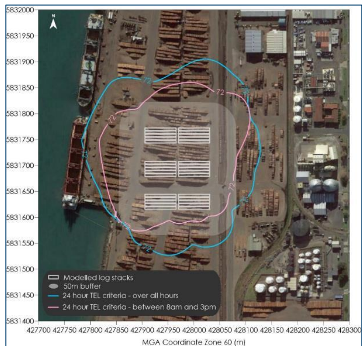
Figure 4-48: Maximum predicted EDN concentrations ( \mu\text{g}/\text{m}^3 ) - Thirty log stacks scenario (over a 6-hour period), 24-hour averages, 500ppm with ventilation across all hours and between 8am and 3pm
