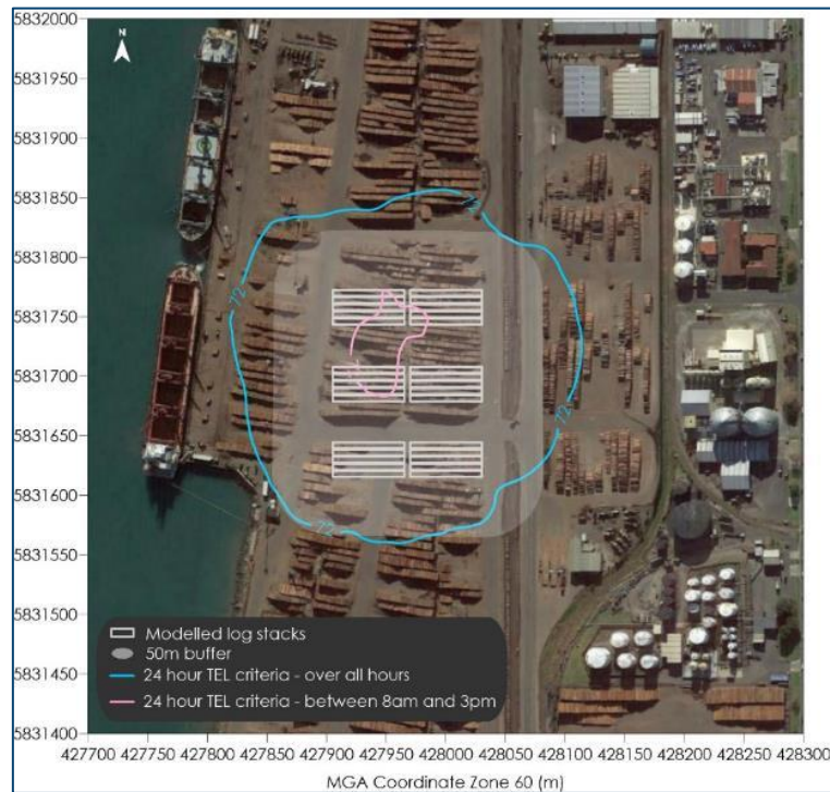
Figure 4-45: Maximum predicted EDN concentrations ( \mu\text{g}/\text{m}^3 ) - Thirty log stacks scenario (over a 8.5-hour period), 24-hour averages, 500ppm with ventilation across all hours and between 8am and 3pm
