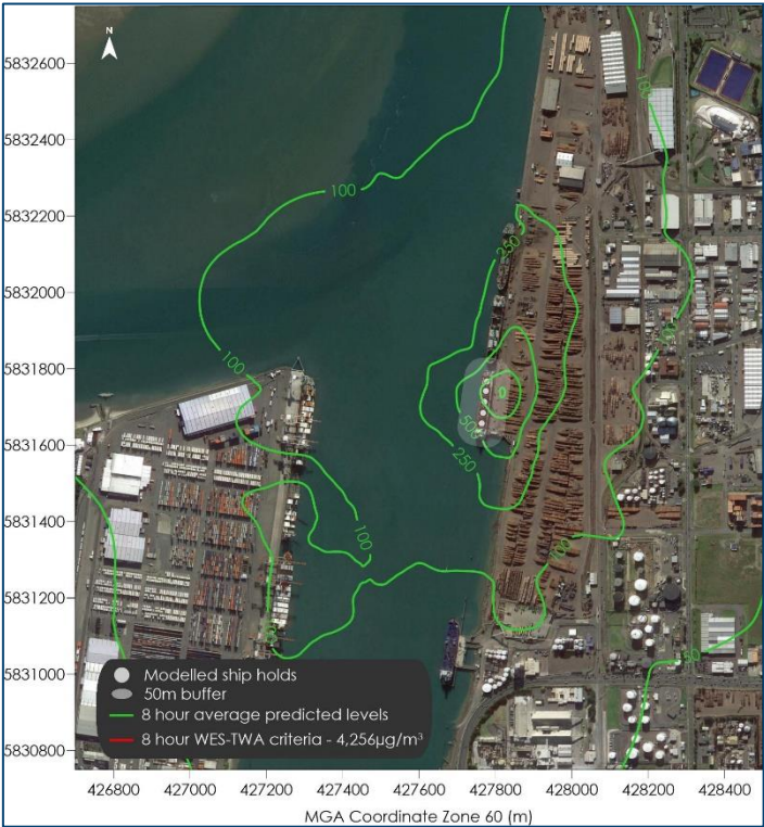
Figure B-55: Maximum predicted EDN concentrations ( \mu\text{g}/\text{m}^3 ) - Ship holds, 8-hour averages, 700ppm
