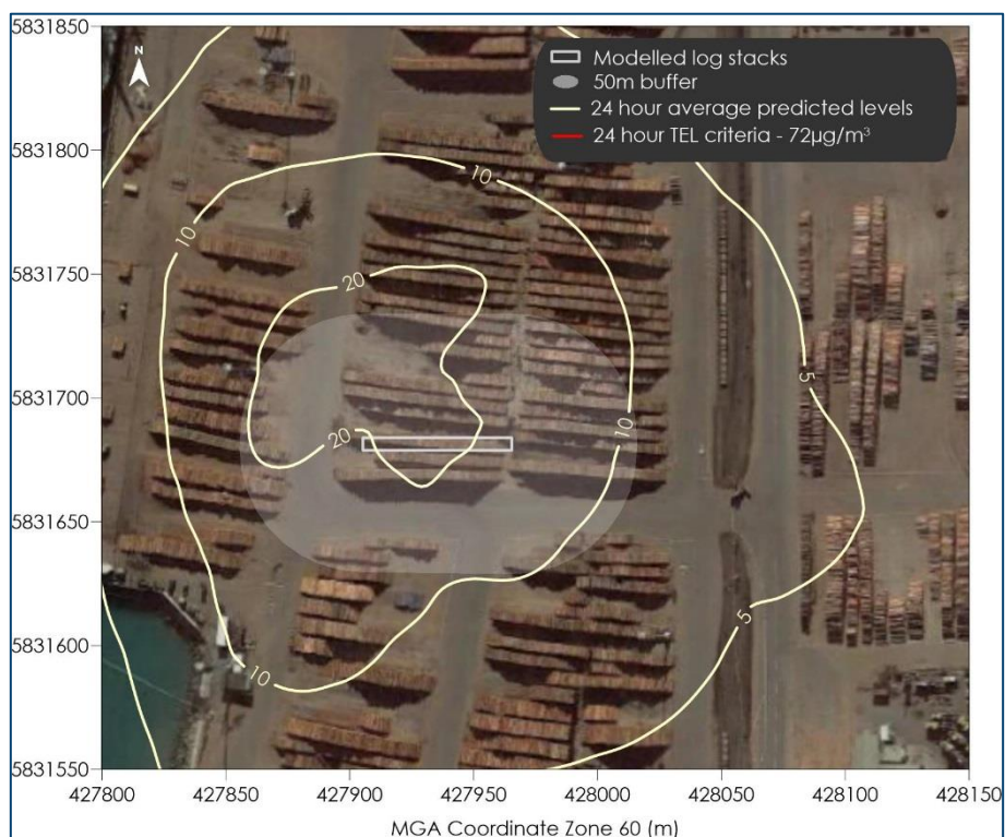
Figure B-8: Maximum predicted EDN concentrations ( \mu\text{g}/\text{m}^3 ) - One log stack scenario, 24-hour averages, 700ppm
