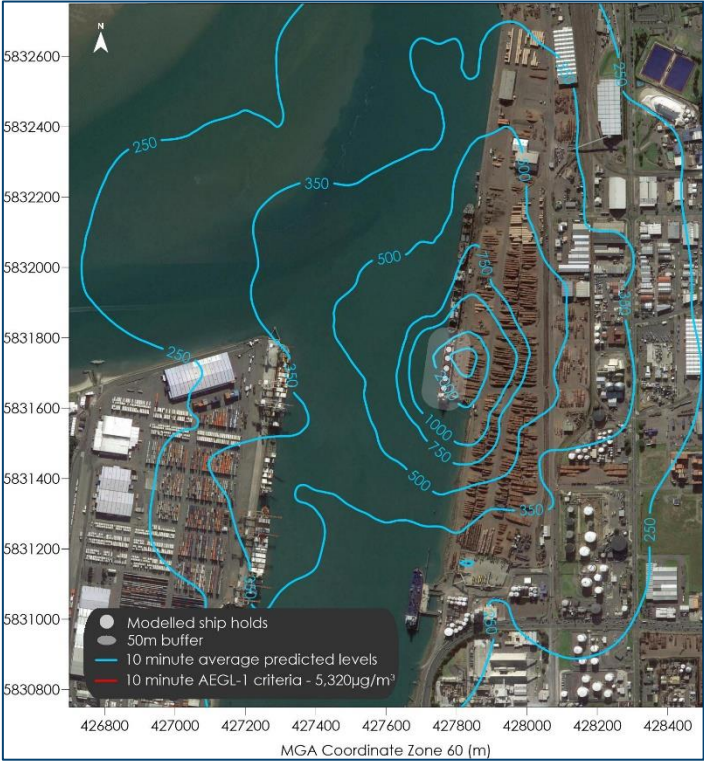
Figure B-49: Maximum predicted EDN concentrations ( \mu\text{g}/\text{m}^3 ) – Ship holds, 10-minute averages, 500ppm
