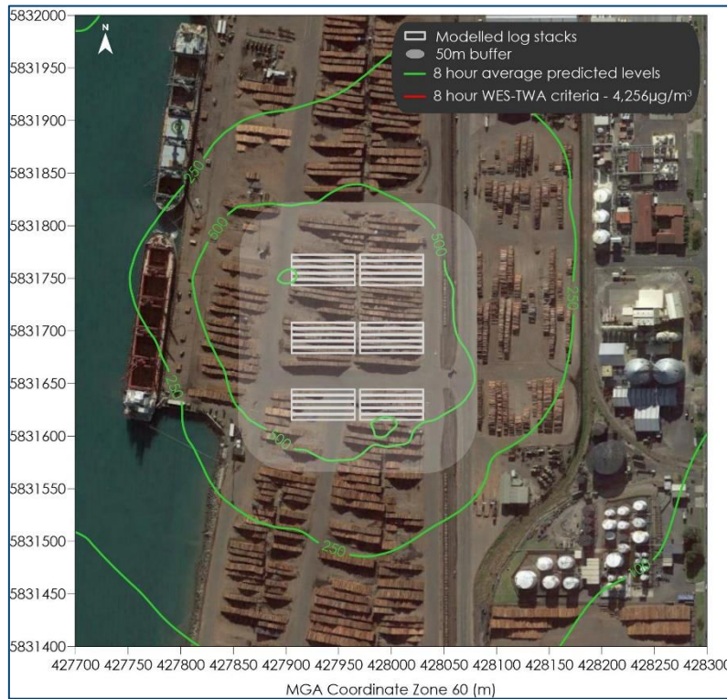
Figure B-47: Maximum predicted EDN concentrations (µg/m³) - Thirty log stacks (over an 8.5-hour period) scenario, 8-hour averages, 1,000ppm
