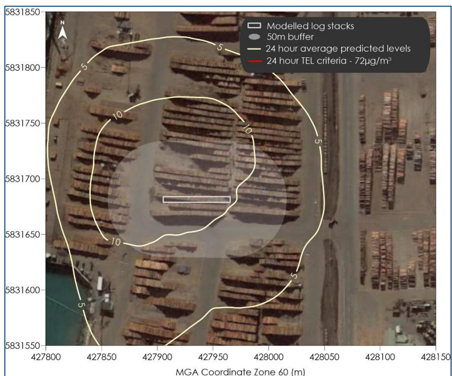
Figure B-4: Maximum predicted EDN concentrations ( \mu\text{g}/\text{m}^3 ) - One log stack scenario, 24-hour averages, 500ppm
