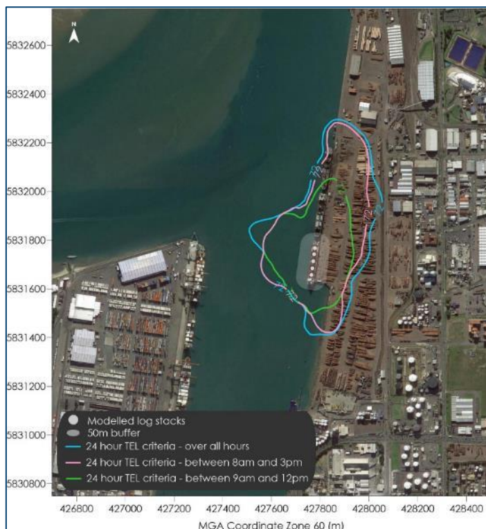
Figure 4-58: Maximum predicted EDN concentrations ( \mu\text{g}/\text{m}^3 ) - Ship holds, 24-hour averages, 700ppm, with ventilation across all hours, between 9am and 3pm and between 9am and 12pm
