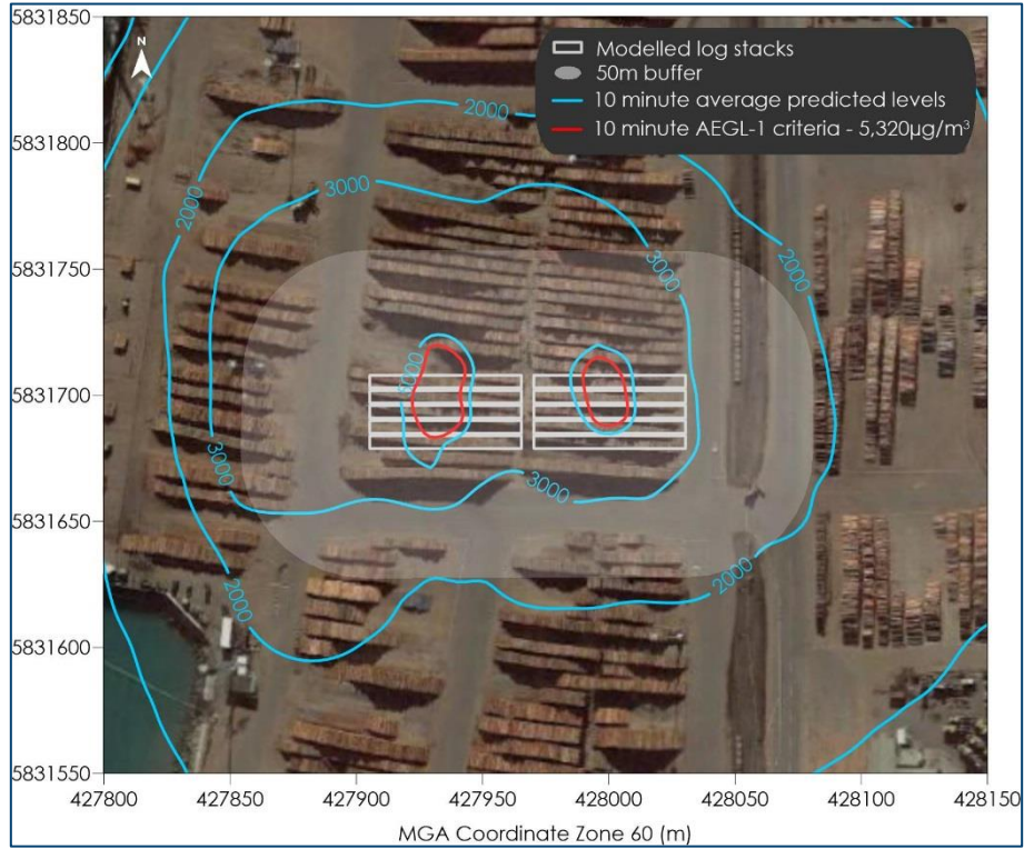
Figure B-33: Maximum predicted EDN concentrations (µg/m3) - Ten log stacks scenario, 10-minute averages, 1,000ppm
