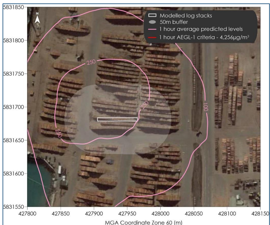
Figure B-2: Maximum predicted EDN concentrations ( \mu\text{g}/\text{m}^3 ) - One log stack scenario, 1-hour averages, 500ppm
