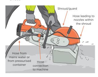
Each part is critical to the system's effectiveness and level of dust control. You can buy a complete on-tool water suppression system or, individual parts of the system to use with your existing tools. Make sure to choose parts that are compatible with your tools. Involve workers in selecting a system that is right for the task.
